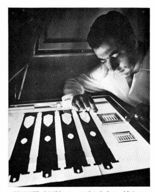
ROLAMITE BANDS are produced from 10-times oversize drawing prepared by Precision Graphics Section 7653-1. The large negatives are photographically reduced to size by Printed Circuitry Lab Section 4221-1 and then the image is transferred to metal and etched in the Rolamite Lab. Tom Cleveland (4222-3) compares negatives with finished set of metal bands.
